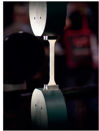
of rotation (to track specimen alignment) during testing. Calibration is digitally embedded but, for extra reassurance, can be checked at any time using the standard traceable gauge block supplied.
