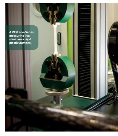
"Our Video Extensometer is perfect for precise, non-contact measurement of specimen strain"
